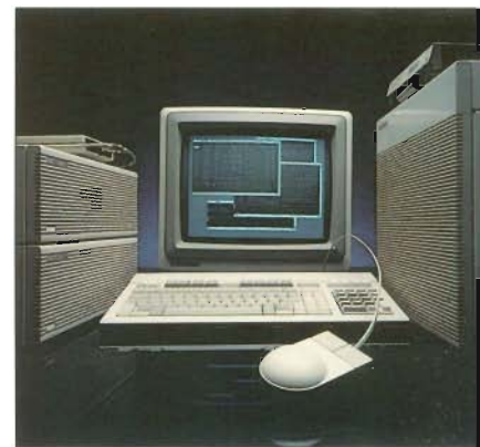
Central to the HP 64000 software design environment is the HP 9000 Series 320 workstations running the HP-UX operating system, high-performance HP peripherals, and advanced software.
